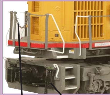
Handrails & Safety Chains MU Cables
