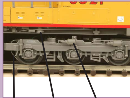
Sanding pipes Bell Brake Cylinders & Air Lines
