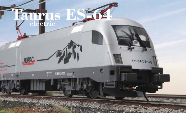
Introduced to the European market in 2000, the Taurus ES 64 U2 Electric was developed as a universal electric locomotive, topping out at a speed of 230km/h. This multipurpose engine has become one of the most influential representatives of Dispolok GmbH, a Siemens Transportation System subsidiary, making leasing options available to a host of different rail operators.
