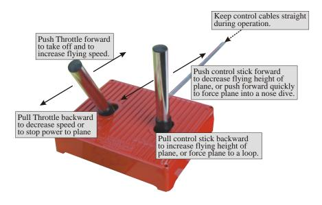
Speed and height of plane in flight are managed by operation of the Throttle and Control Stick on the Airplane's Control Box:
