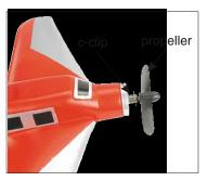
**3.** Attach C-Clip to arm at airplane nose. Push propeller onto shaft.
