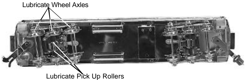
Fig. 3 Lubricating the Passenger Car
