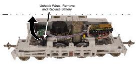
Figure 3b. Replacing the Battery
