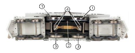
Figure 2. Lubrication Points on the Locomotive
