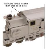
Figure 3a. Screws to Remove to access the inside of the engine.
