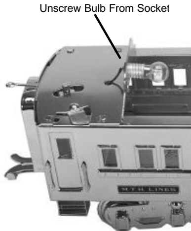
Fig. 5 Unscrewing the Bulb from its Socket
