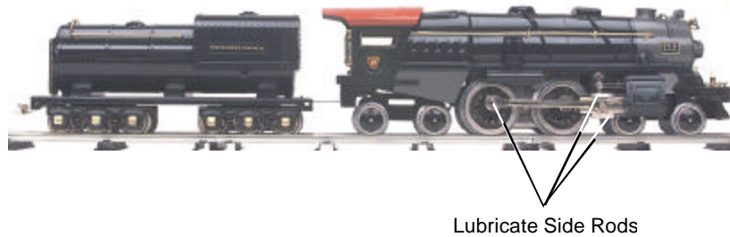
Figure 2: Lubricating Side Rods
