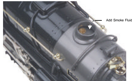
Figure 14: Filling The Smoke Unit
