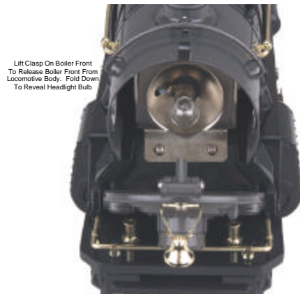
Figure 11: Replaceable light bulb locations
