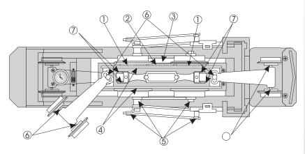
Figure 7: Lubricating The Locomotive Chassis
