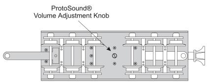
Figure 5: Adjusting The ProtoSound® Volume
