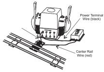
Figure 6: Wiring Up A Bell Button
