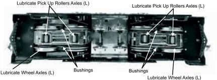
Figure 1. Lubrication Points on the Locomotive
