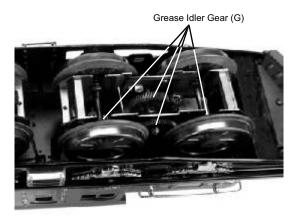
Figure 3 Grease Idler Gears
