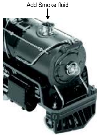
Figure 3: Adding Smoke Fluid
