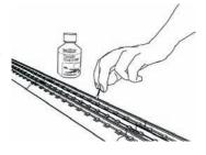
transformer and wipe the rails of the track, turning the rag frequently to ensure that you are using clean cloth on the rails. Thereafter, keep an eye on the track and clean it when it gets dirty to ensure good electrical contact and to lengthen the life of the tires.
