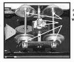
Lubricate pickup rollers, where axle meets wheel and where axle meets truck side.
