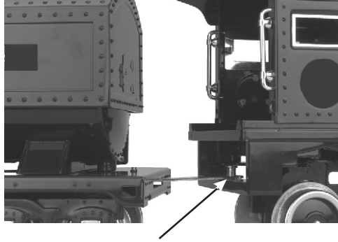
Connect Draw Bar Here As Shown
