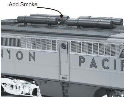
Adding Smoke Fluid
