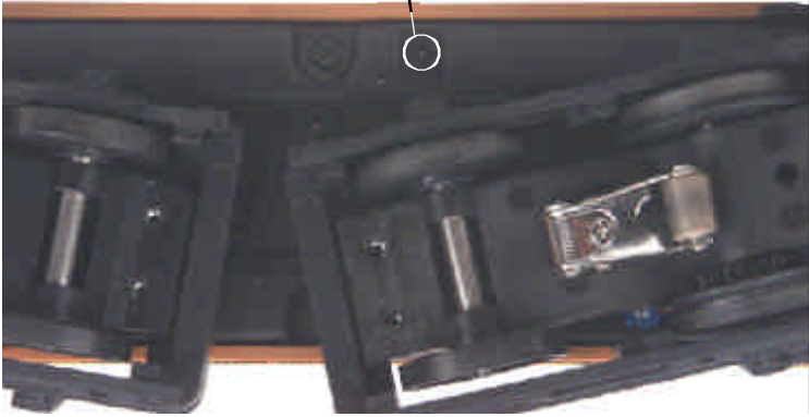
Figure 7: Battery Charger Port
