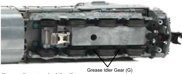
Figure: Greasing the Idler Gears
