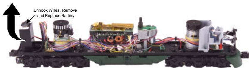
Figure 10. Replacing the Battery
