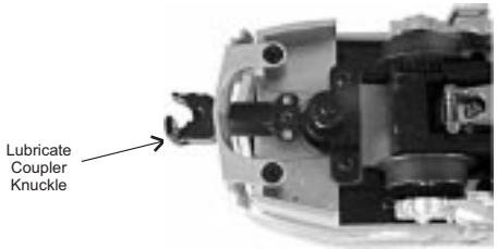
Figure 3: Lubricating The ProtoCoupler Knuckle
