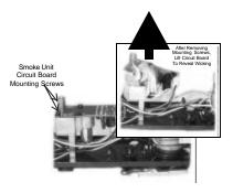
Figure 2: Inspecting The Smoke Unit
