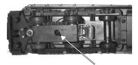
Truck Block/Motor Mount Attachment Screw Figure 7: Lubricate The Tender Chassis Trucks
