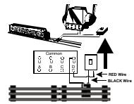
Figure 5: Wiring Up A Bell Button
