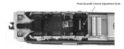
Figure 4: Adjusting The ProtoSound® Volume and selecting the ProtoCoupler
