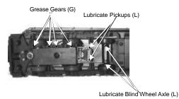
Figure 6: Lubricating The Locomotive Chassis
