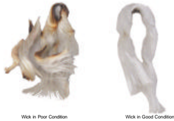
Figure 7. Examples of a wick in poor condition and in good condition.
