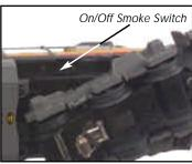
Figure 6 - Smoke Unit On/OffSwitch
