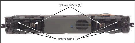
Figure 2 - Lubrication Points on the Engine
