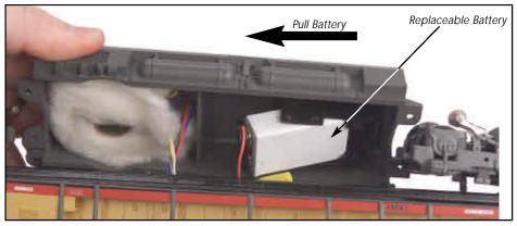
Figure 11- Replacing the Battery
