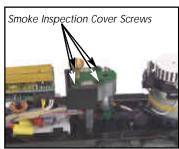
Figure 7 - Smoke Unit Inspection Cover
