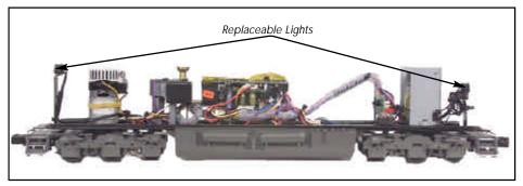
Figure 8 - Replacing the Headlights
