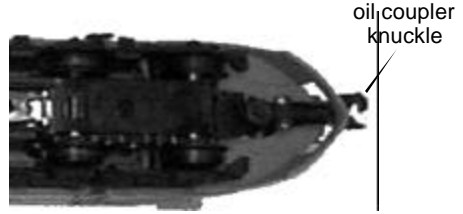
Figure 4: Lubricating The ProtoCoupler Knuckle
