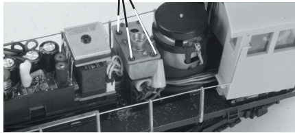
Inspection Cover Screws
