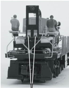
1) Remove Screws from back end
