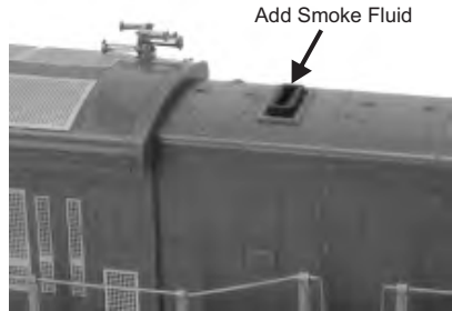
Figure: Adding Smoke Fluid
