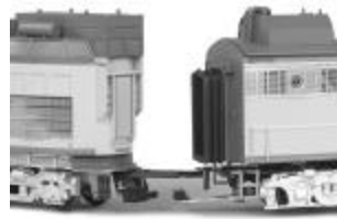
Figure 2: Connecting the A and B Units together by aligning the draw bar to the pin and also align connectors to each other. Then press the two units together.
