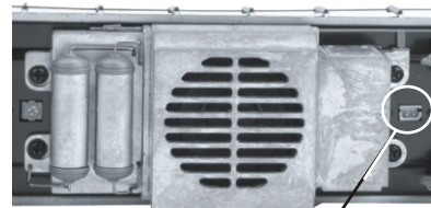
Battery Charger Port
