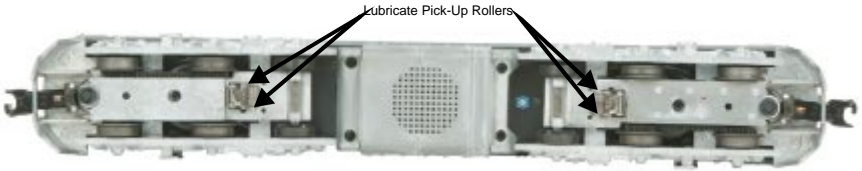
Figure 1. Lubrication Points on the Locomotive
