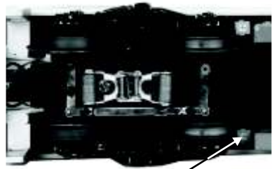
Smoke Unit Control
