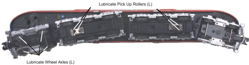
Figure 1. Lubrication Points on the Locomotive
