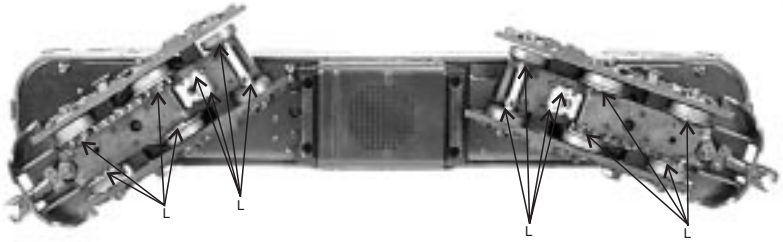
Figure 7: Lubricating The Truck
