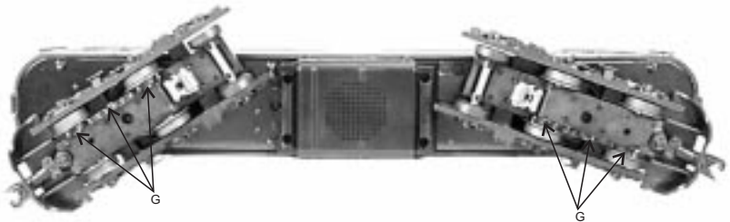
Figure 8: Greasing The Power Trucks
