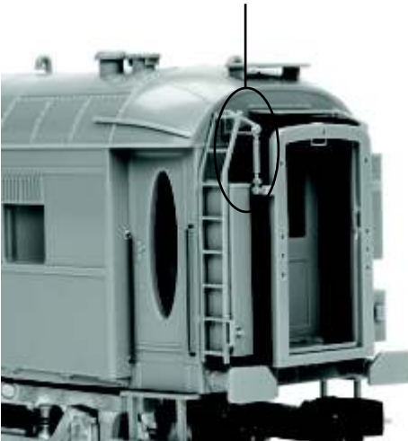
Attach the diaphragm supports to the diaphragm.
