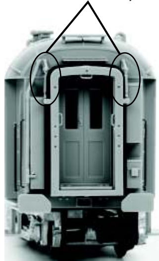
Apply diaphragm supports to the ends of the body
