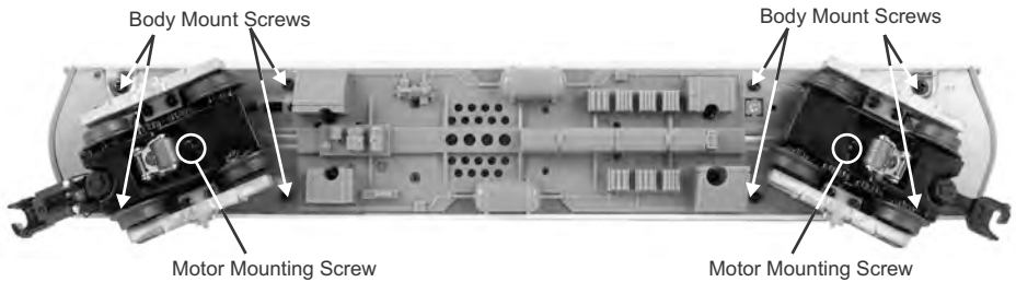
Figure: Body Mount and Motor Mount Screws
