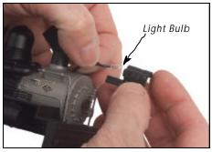
Figure 8 - Replacing the Headlight
