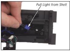
Figure 9 - Replacing the Headlight
