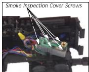
Figure 6 - Smoke Unit Inspection Cover
