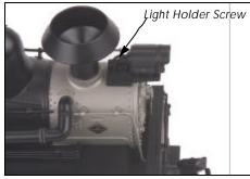
Figure 7 - Replacing the Headlight
