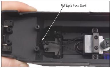
Figure 7 - Replacing the Headlight
