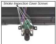
Figure 6 - Smoke Unit Inspection Cover
