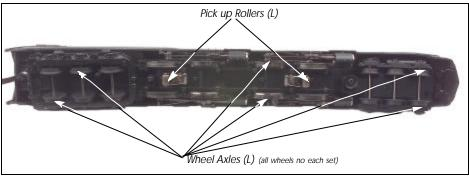
Figure 2 - Lubrication Points on the Engine
