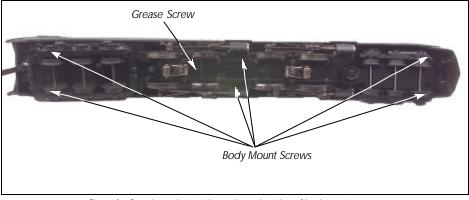
Figure 3 - Greasing points on the engine & location of body mount screws
