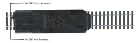
Proper 2-Rail polarity wiring and locomotive orientation (Reference photo)
