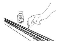
Unplug the transformer and wipe the rails of the track, turning the rag frequently to ensure that you are using clean cloth on the rails. Thereafter, keep an eye on the track and clean it when it gets dirty to ensure good electrical contact and to lengthen the life of the tires.
