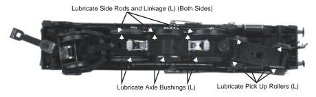
Lubrication Points on the Locomotive
