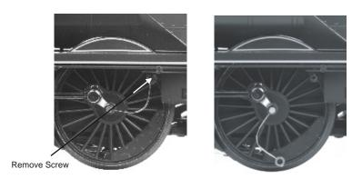
You must remove the truck detail in order to remove the body from the chassis. (shown above)
