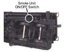
Figure 4. Smoke Unit ON/OFF Switch
