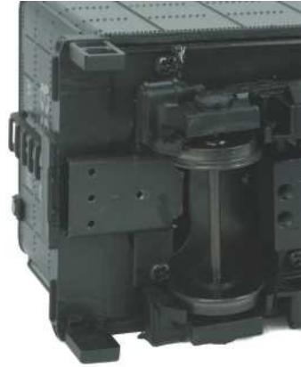
Figure 5: Pre-drilled Kadee® Coupler mounting holes
