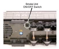
Figure 4. Smoke Unit ON/OFF Switch
