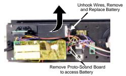
Figure 11. Replacing the Battery
