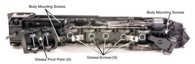
Figure 7a. Location of Body Mount Screws and Greasing Points on the Locomotive
