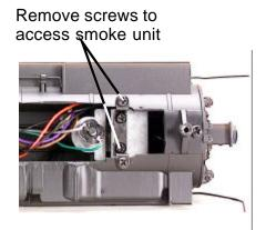
Figure 5a. Accessing the Smoke Unit
