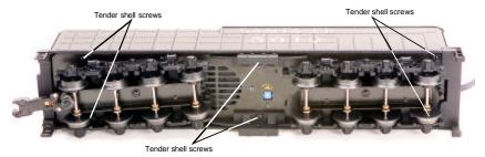
Figure 9. Screws to remove the tender shell
