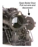
Figure 8a. Replacing the Headlight
