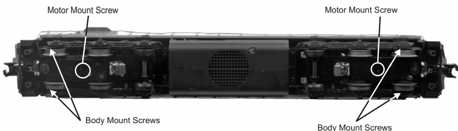
Figure 6: Body Mount Screws
