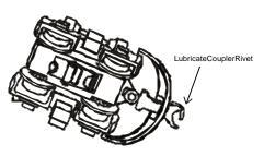
Figure 3: Lubricating The ProtoCouplers
