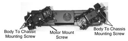
Figure 7: Lubricate The Tender Chassis Trucks
