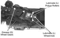
Figure 6: Lubricating The Locomotive Chassis
