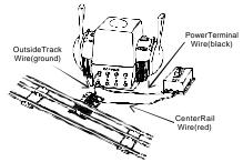
Figure 5: Wiring Up A Bell Button
