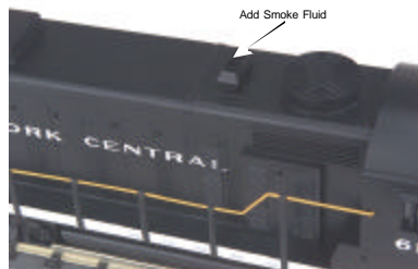
Figure 10: Adding Smoke Fluid
