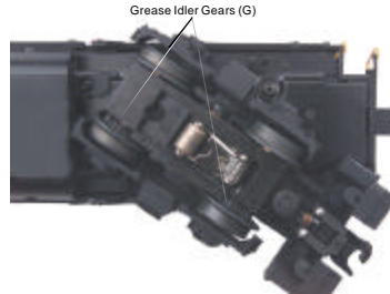
Figure 6: Greasing The Idler Gears
