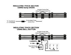
operator attempt to have the rear roller of the car leave the insulated track section shortly after the 3 second push of negative DC has been received by the ProtoSound® module inside the Trolley car. This way, when TAS has
