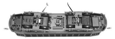
Figure 3: Lubricating The Locomotive Chassis
