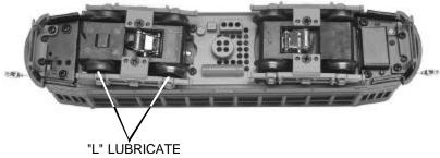
Figure 4: Lubricate The Truck Bushings
