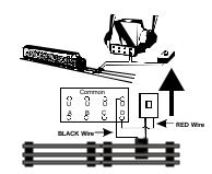
Figure 2: Wiring Up A Bell Button
