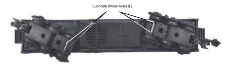
Figure 1. Lubrication Points on the Locomotive
