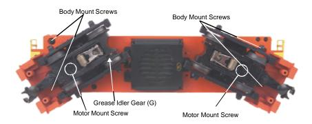
Figure 3. Body Mount Screws and Greasing Points.
