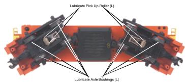
Figure 2. Lubrication Points on the Engine
