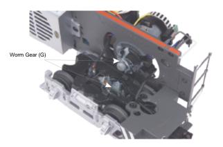
Figure 3a. Grease the Worm Gear
