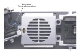
Figure 1. Location of the Loco-Sound Volume Adjustment Knob
