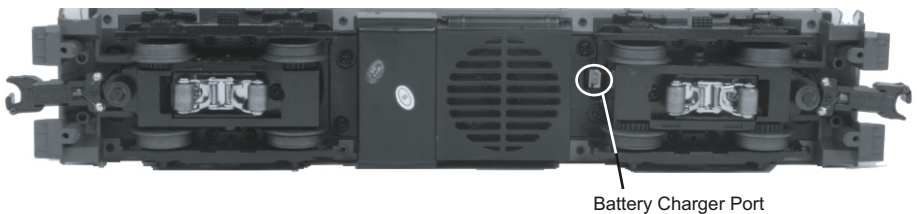
Battery Charger Port Location
