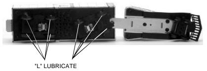
Figure 4: Lubricate The Truck Bushings
