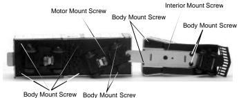
Body Mount Screw Body Mount Scree Figure 5: Removing The Body From The Chassis
