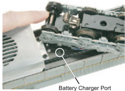
Leave the engine in neutral with track voltage at 10-12 volts for 6-7 hours so the battery can fully recharge (if your engine has a smoke unit, be sure it is turned off).
