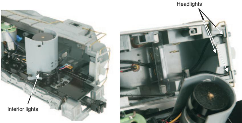
Figure 7. Replacing the Light Bulbs
