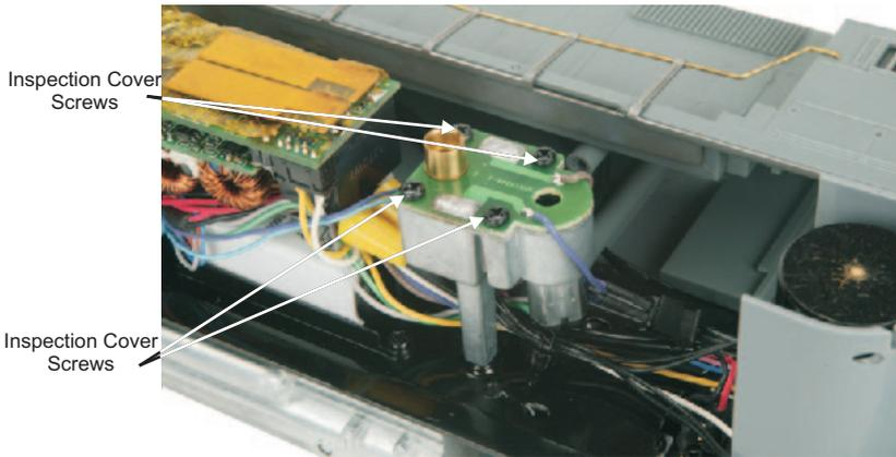
*Figure 9. Inspecting the Smoke Unit Wick*
