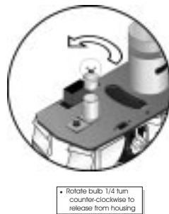
Figure 15: Removing the locomotive headlight bulb.
