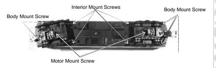
Figure 5: Removing The Body From The Chassis
