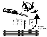
Figure 2: Wiring Up A Bell Button
