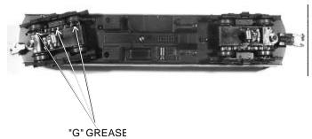
Figure 4: Lubricate The Truck Bushings
