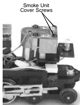
Figure 12. Inspection Cover Screws
