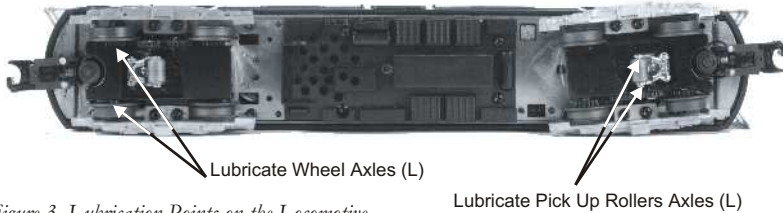
Figure 3. Lubrication Points on the Locomotive.
